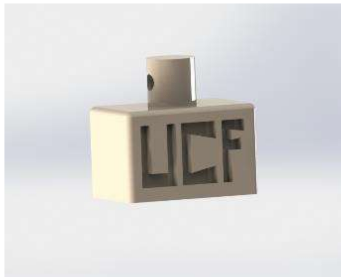
Figure 37: shows a CAD version of the 4 servo housing that will be put on the 2 front and 2 back tires for maneuvering abilities.
