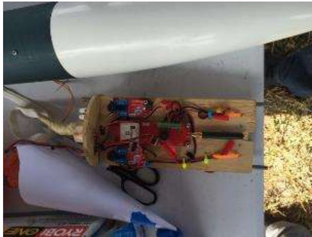
Figure 4: Finished Avionics Bay Front
