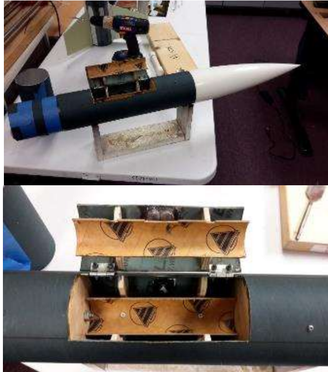
Figure 6: Finished payload section
