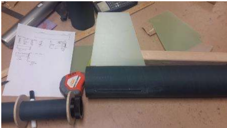
Figure 2: test fitting positioning of rings, fins, and retainer
